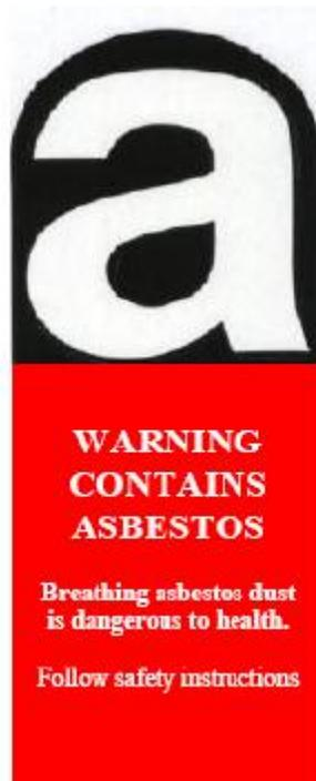
*Asbestos warning label to be clearly displayed on double polythene bags*
